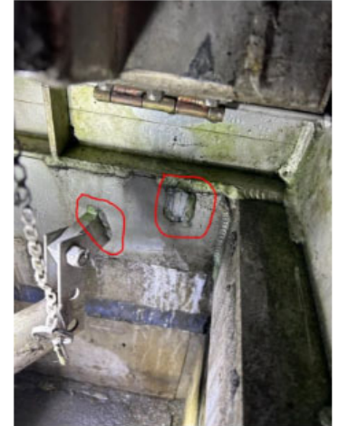
Lift Assist Spring Cylinder Broken Weld
